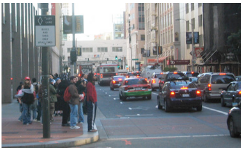
As congestion grows on a street, violations of the bus-only lane increase. In the left photo, three vehicles are violating the bus-only lane. None are in the right photo.
